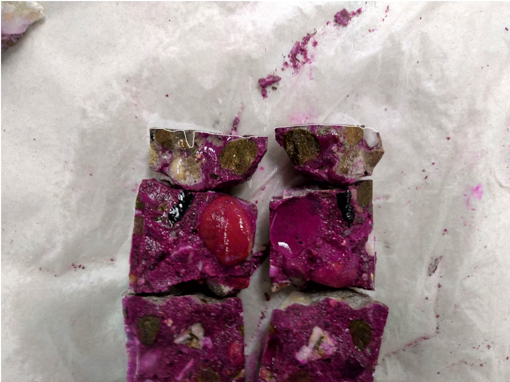
Figure E.43: Carbonation front C1-23.
