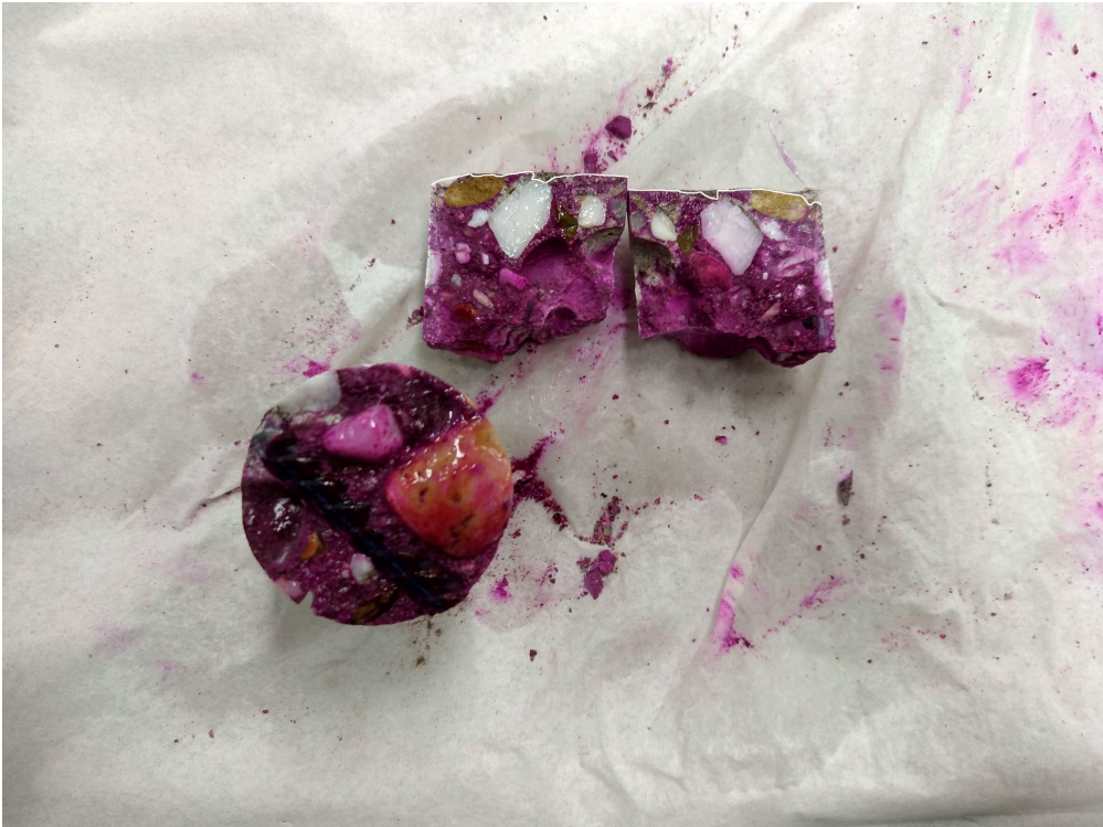
Figure E.35: Carbonation front C1-1.
