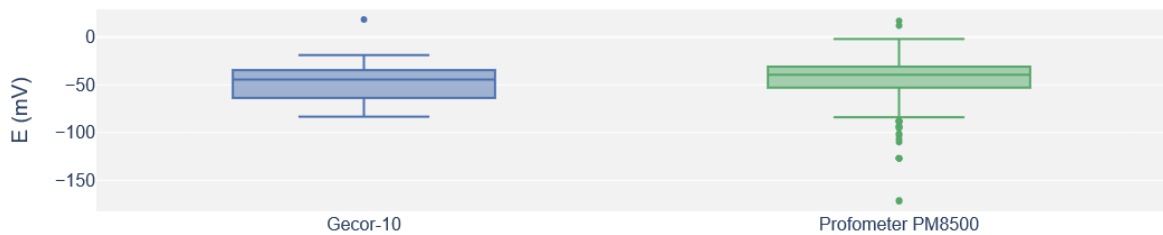
Figure 5.13: Boxplots of the half-cell potentials measured on the support beam using the Gecor-10 and Profometer PM8500.
