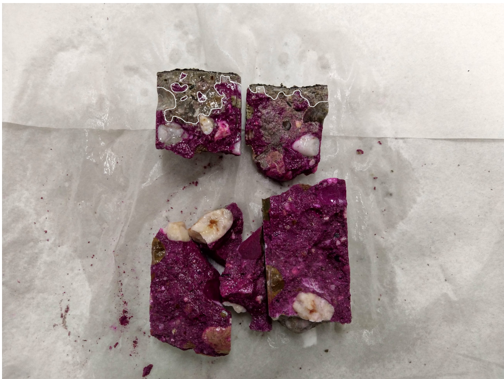
Figure E.34: Carbonation front C6.
