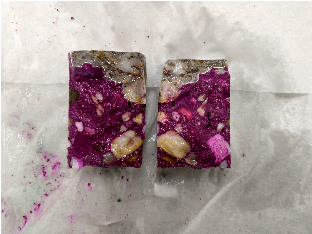
Figure E.36: Carbonation front C2-1.
