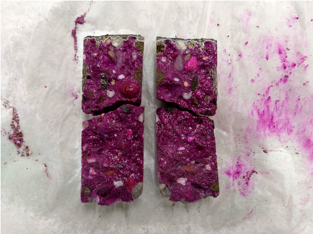
Figure E.31: Carbonation front C3.
