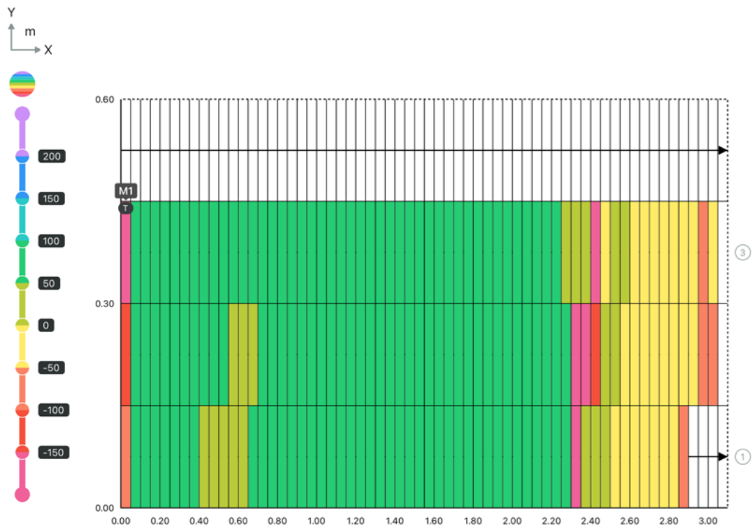
Figure F.14: Beam 1 east face half-cell potential map (2).
