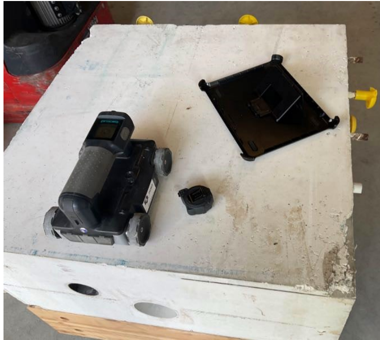
Figure 2.13: Concrete testing block at Newa HQ and Screening Eagle's GP8000.
