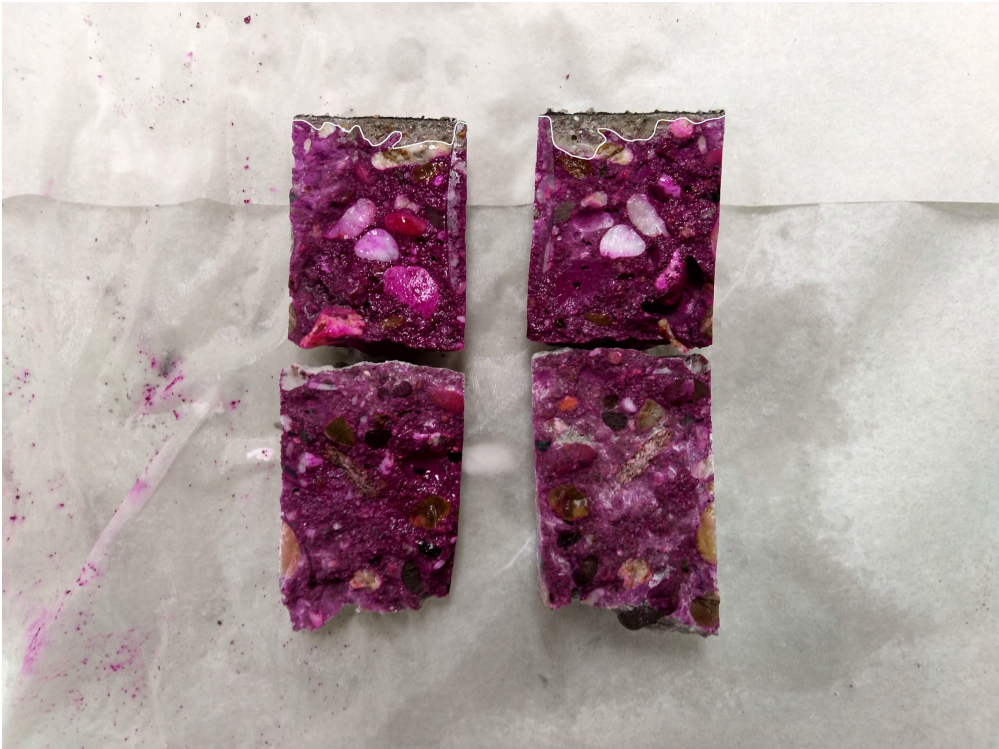
Figure E.32: Carbonation front C4.
