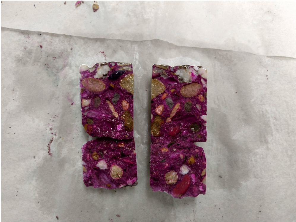
Figure E.37: Carbonation front C1-7.
