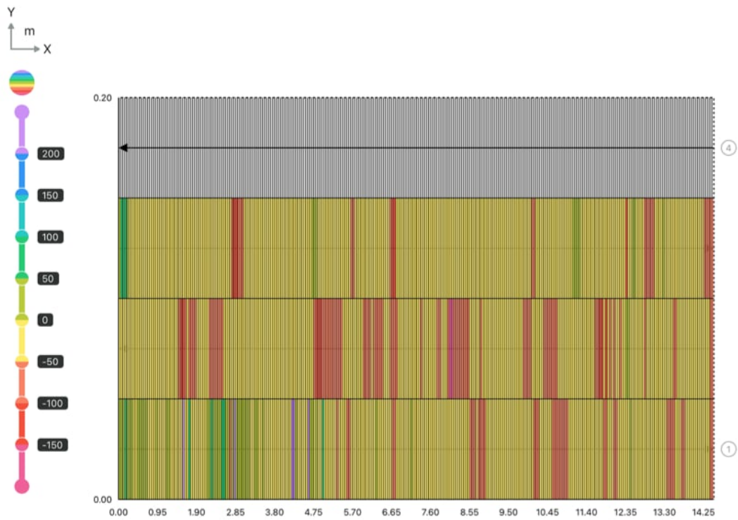
Figure F.12: Support beam half-cell potential map (2).
