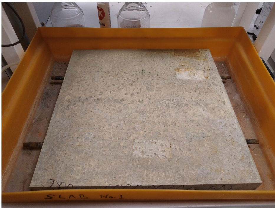
Figure G.1: Reinforced concrete OPC slab pre-wetting.
