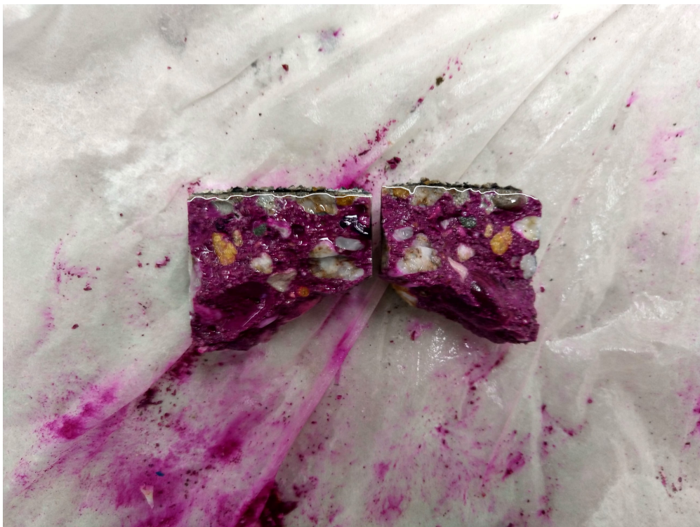
Figure E.30: Carbonation front C2.
