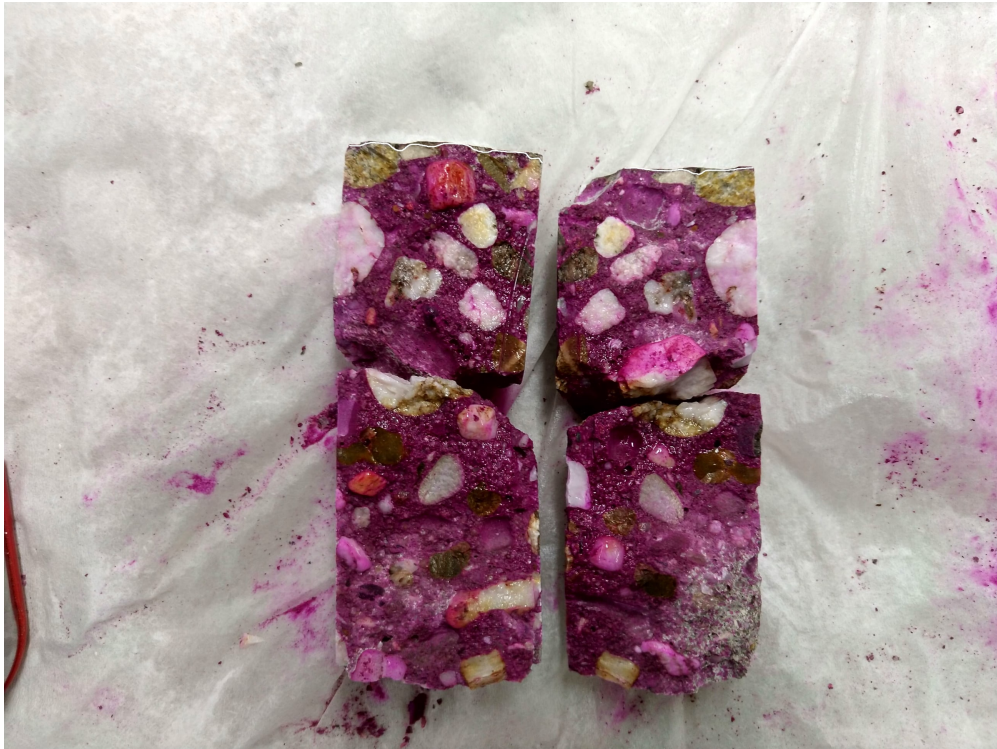
Figure E.41: Carbonation front C1-18.
