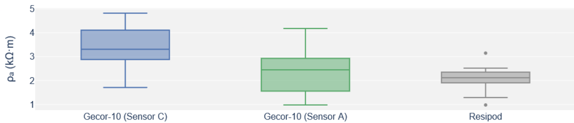
Figure 5.15: Boxplots of the resistivity measured on the support beam using the Gecor-10 and Resipod.
