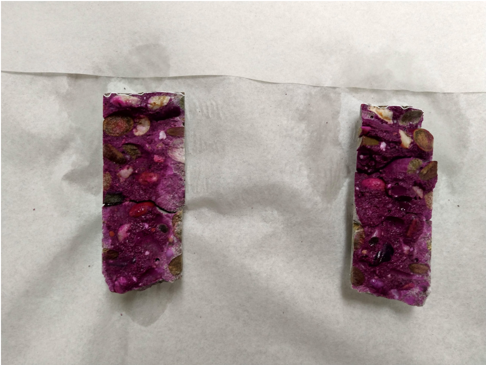
Figure E.44: Carbonation front C2-23.
