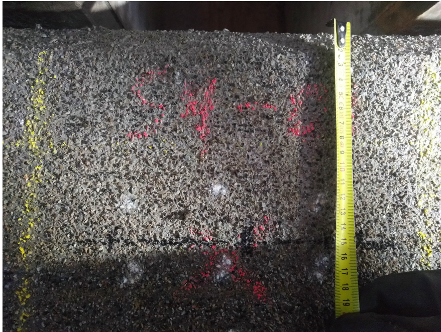
Figure 4.6: Distance of 15 cm from the UPV centerline to the top of the support beam.
