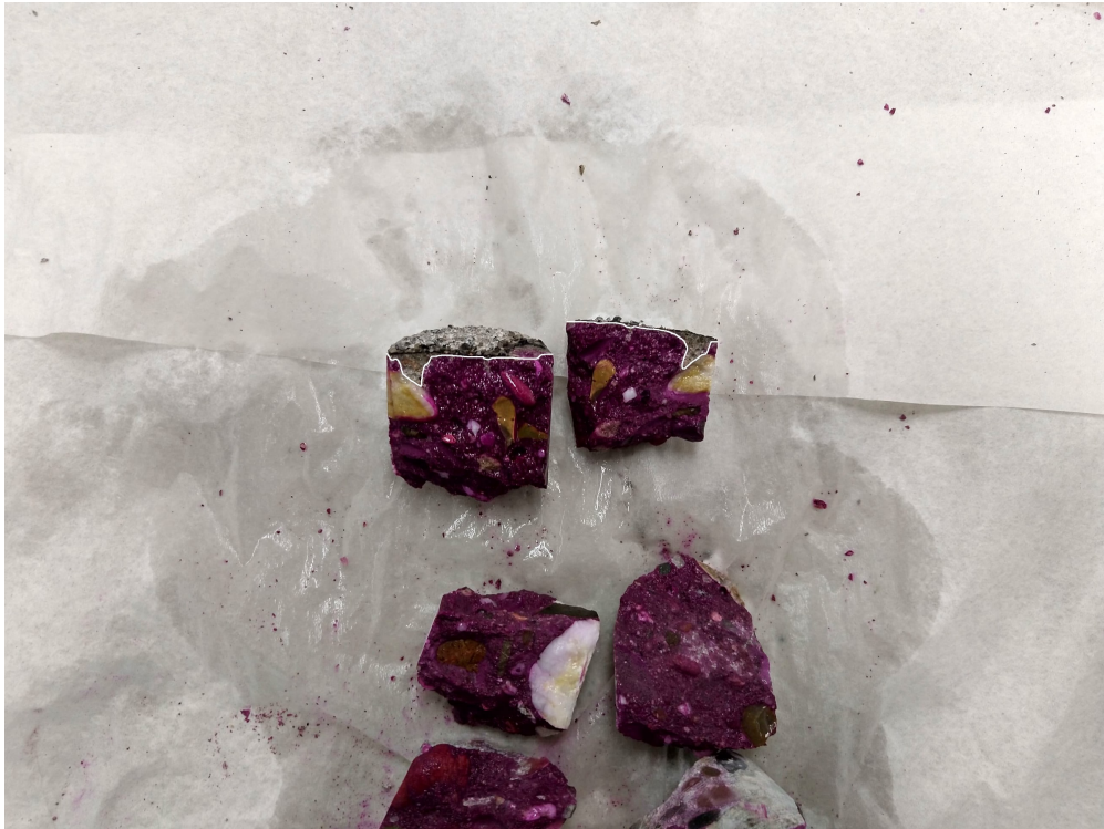
Figure E.29: Carbonation front C1.
