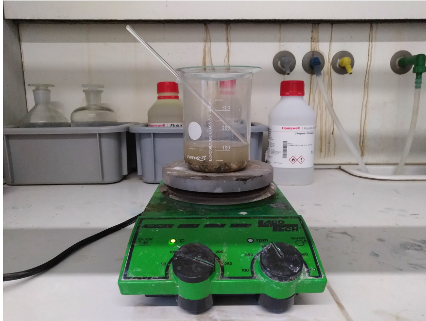
Figure 4.17: Boiling the sample in 4M nitric acid.
