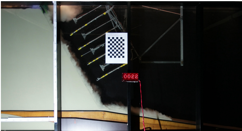
Figure 3.7: Generation of a plume of sand particles upon the removal of the confining wall during the 60^\circ experiment. The digital clock refers to the time of the UVP measurements and the checkerboard was used in combination with the horizontal and vertical rulers for camera calibration.
