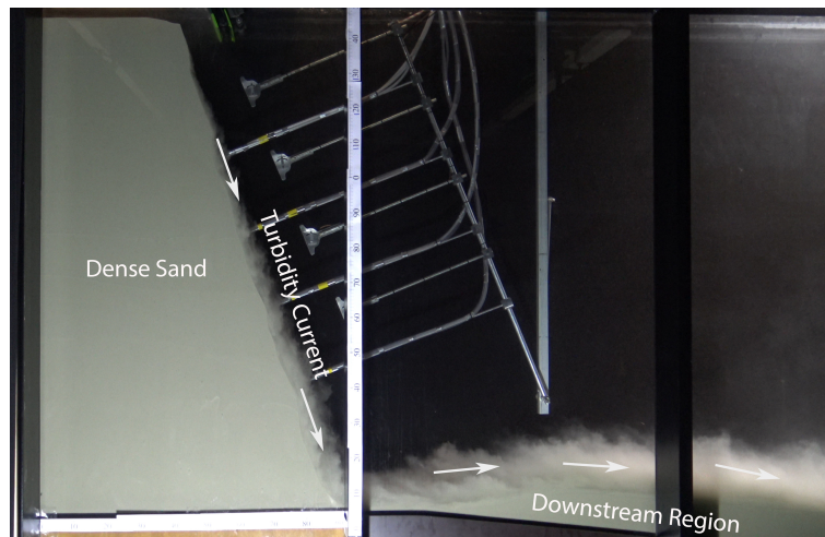
Figure 3.12: The experiment in progress: the turbidity current and the deposition of sediments in the downstream region.
