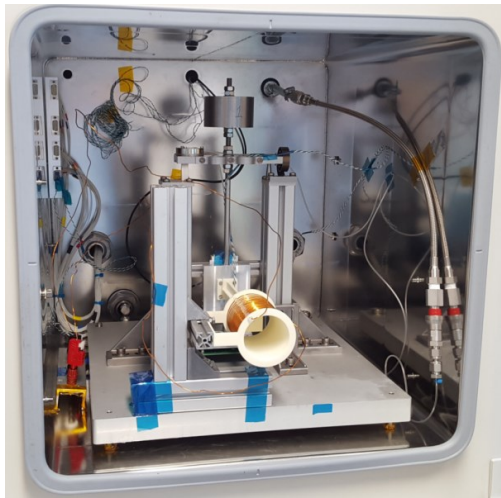
Figure 15. AE-TB-5m test stand inside a vacuum chamber
