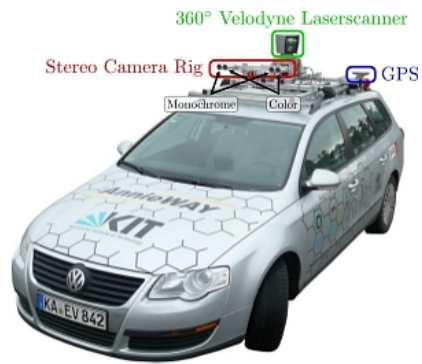
Figure A.1: MMS employed for the acquisition of KITTI dataset. Acquired from Geiger et al. (2012).
