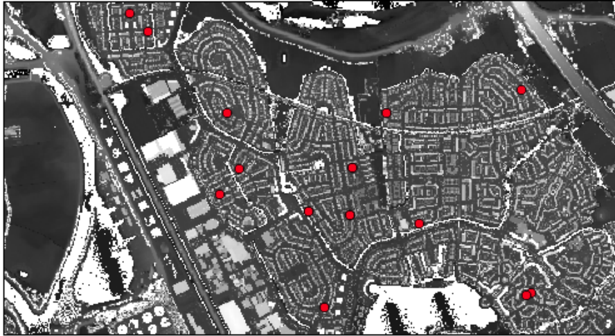
Figure 8.2: The AHN layer in QGIS with the red dots representing roofs with PV systems designed with the Solar Monkey software.
