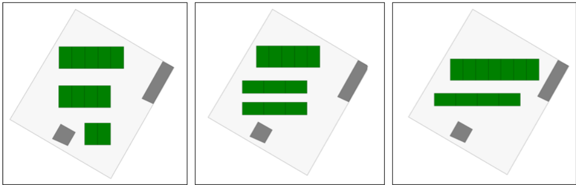
Figure 9.6: Some solutions to a flat roof when placing a limited amount of panels with a south orientation.
