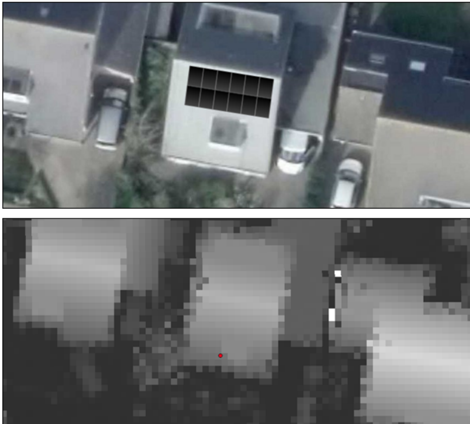
Figure 8.3: A PV system designed with the Solar Monkey software and the corresponding AHN layer.
