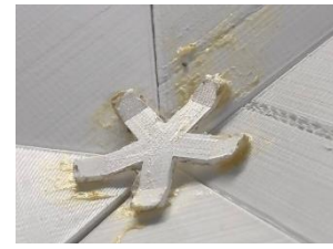
Figure 95 Messy glue test
