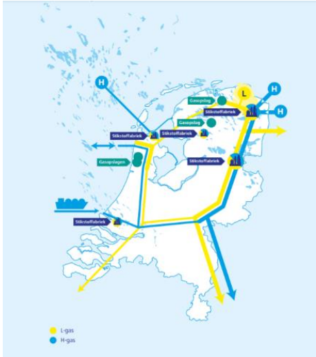
Figure 13: L-gas and H-gas network, from (GasTerra, 2019)
